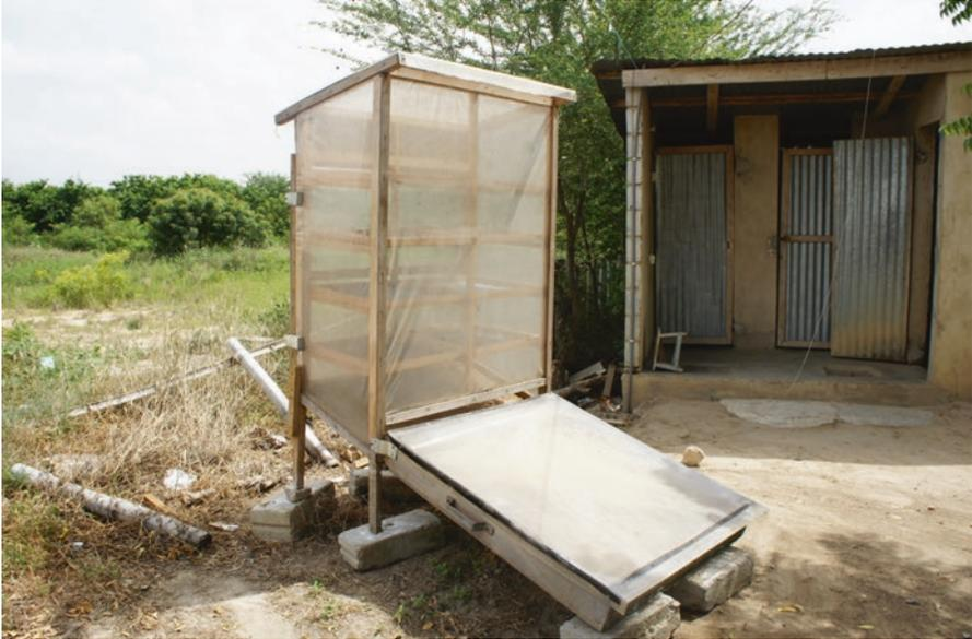
**Fig. 2** Solar dryer used to dry fly larvae in Ghana (Photo: M. Kenis)
